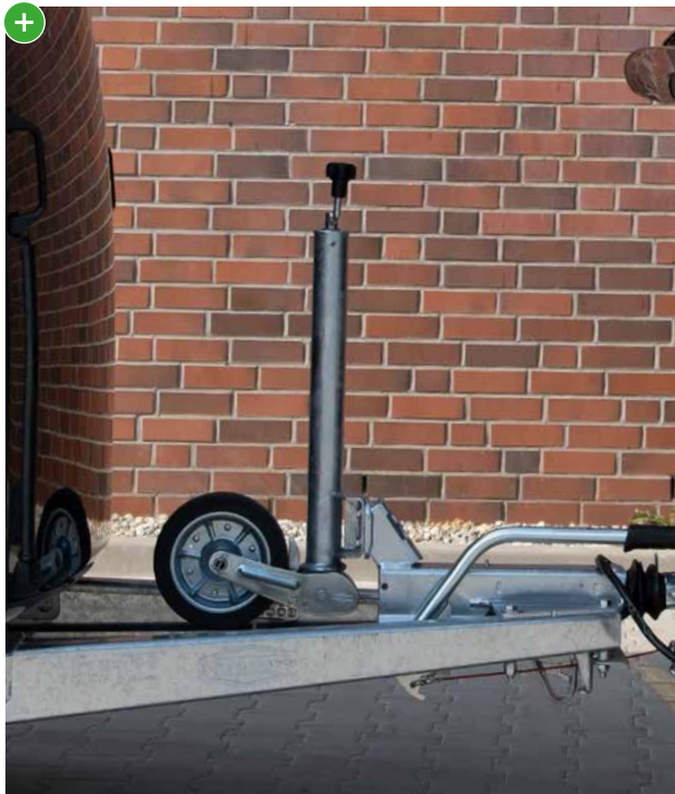
Solid, automatic jockey wheel with user-friendly plastic handle for quick cranking up and a secure stand (single-axle models with robust jockey wheel).
