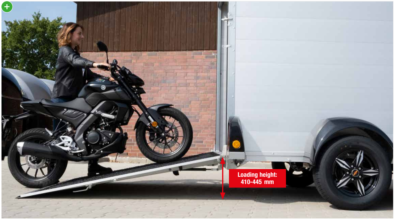
Low loading height and flat ramp for particularly easy loading and unloading. Thanks to the F-version, the models have a particularly low loading height of 410-445 mm. The exact values can be found in the technical data on page 16.
