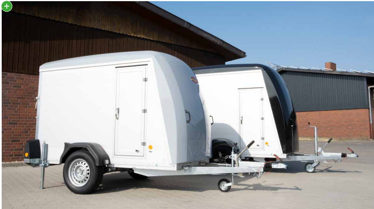
Robust body with polyester bow and roof in 2 sizes as a design feature with high utility advantage: Designed for large transport volume, with storage areas on the front inside and the aerodynamic shape for less fuel consumption. The superstructure made of particularly robust, double-walled profiles of anodised aluminium for maximum stability and durability.
