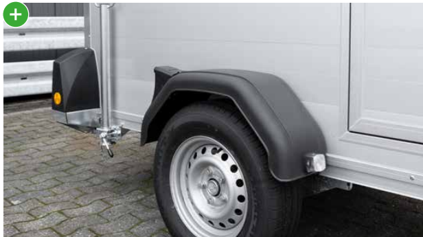
Plastic mudguards and light box cover in an attractive design. Among other things, to protect the lighting for even more durability and practical, e.g. for stowing the wheel chocks and as a storage surface.
