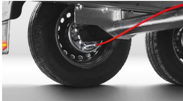
Maintenance-free rubber spring axle with independent wheel suspension for permanently excellent suspension and ride comfort.
