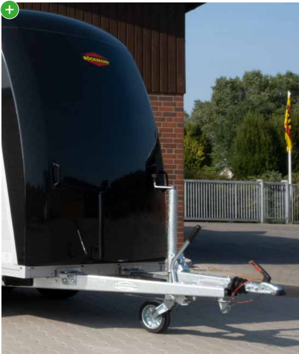
Bolted V-drawbar V-drawbar bolted directly to the frame and a bolted chassis - for excellent ease of maintenance and service.
