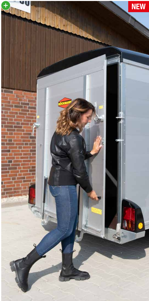
Door-ramp combination The perfect transport solution for flexible use as a door or drive-on ramp. Particularly sturdily constructed and lockable, with robust angle lever lock and particularly easy to operate with the handle in the right place (alternatively available with wing door, see accessories).
