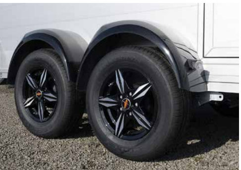
Polyester fenders in an appealing design, high quality and particularly impact-resistant, in anthracite-metallic.
