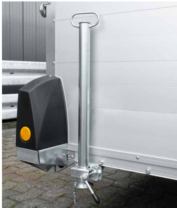
Sliding supports The sliding supports are bolted to the frame and provide a safe stand. Standard on the single-axle models.
